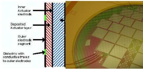
**Fig. 1.** Left: Cross-sectional schematic of the PZT cell structure. Right: A photo of a flat Corning Eagle™ test mirror with deposited PZT film and a pattern of the independently addressable electrodes.
