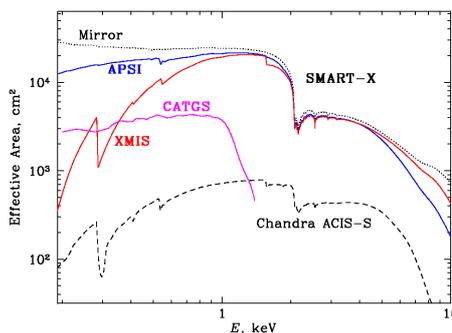
**Fig. 2.** Effective area of the *SMART-X* optics and science instruments.
